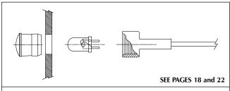
Install lens through panel, insert LED into connector, press connector onto lens to complete installation.
