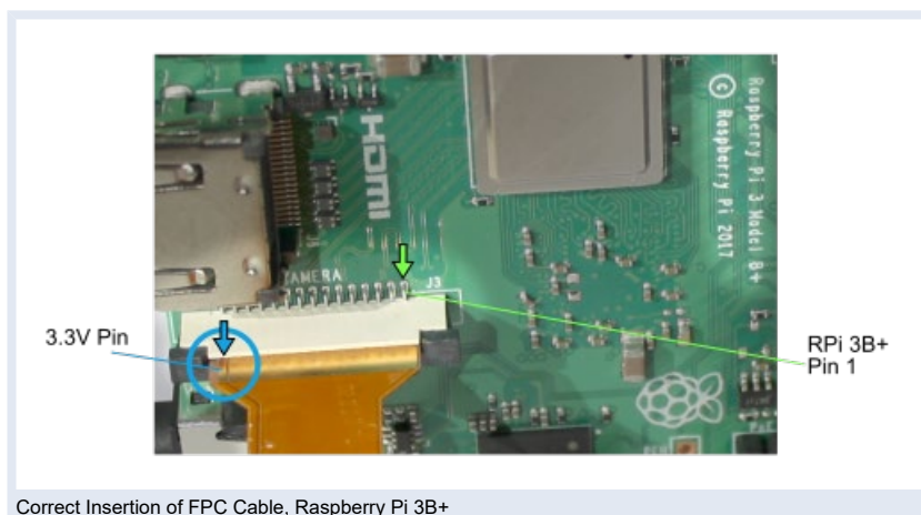
Correct Insertion of FPC Cable, Raspberry Pi 3B+
