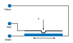
The voltage varies according to the position of the presser on the deformable membrane.
