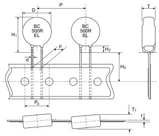
Taping on reel with F = 7.5 mm and 10.0 mm wire pitch, spacing paper tape and foam separator tape used on reel.
