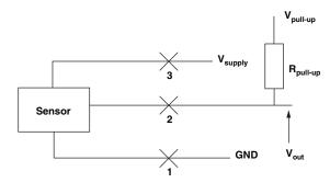
$\rm V_{pull-up}$  can be independent to  $\rm V_{supply}$
