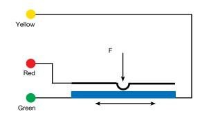
The voltage varies according to the position of the presser on the deformable membrane.
