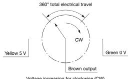
Voltage increasing for clockwise (CW) direction viewed from control shaft side
