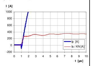
Fast increasing currents (higher than the specified  $I_{\text{\tiny p,max}}), \text{ e.g.}$  in case of a short circuit, can be transmitted because the currents are transformed directly and be limited by diodes only.
