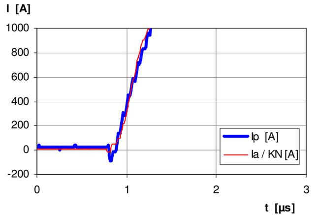
Fast increasing currents (higher than the specified  $I_{p,max}$ ), e.g. in case of a short circuit, can be transmitted because the currents are transformed directly.
