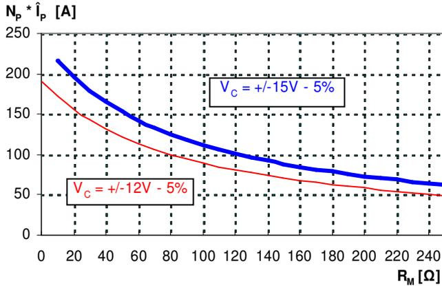
**Maximum measuring range ( $\mu\text{s}$ -range) <sup>1)</sup>**
