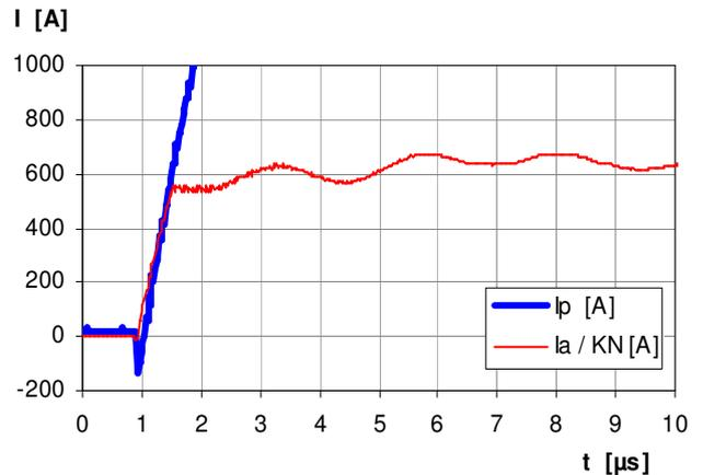
Fast increasing currents (higher than the specified  $I_{p,max}$ ), e.g. in case of a short circuit, can be transmitted because the currents are transformed directly and be limited by diodes only.
