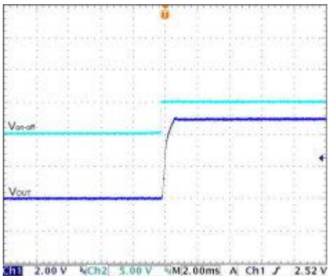
Using ON/OFF Voltage Start-Up and V_{out} Rise Characteristic V_{in} = V_{in\,nom} , Full Load
