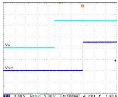
Typical Input Start-Up and Output Rise Characteristic
