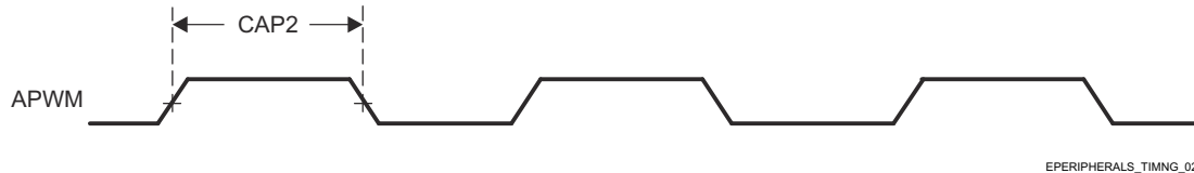
Figure 6-45. eCAP Output Timings
