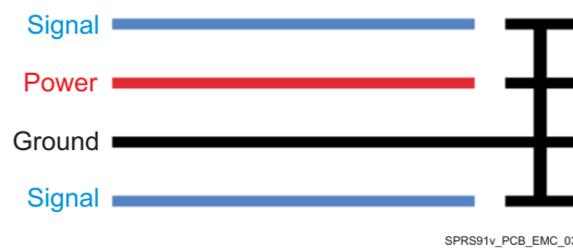
Figure 8-13. Guard Ring Routing
