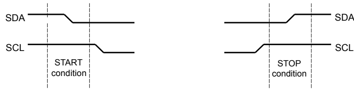
Figure 15-3. START and STOP Conditions
