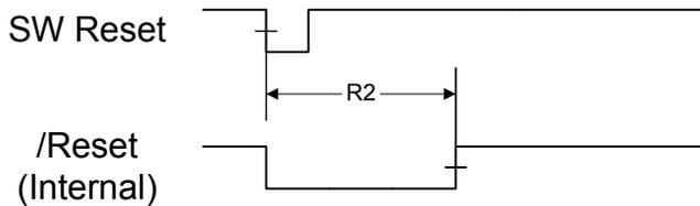
**Figure 25-12. Watchdog Reset Timing**
