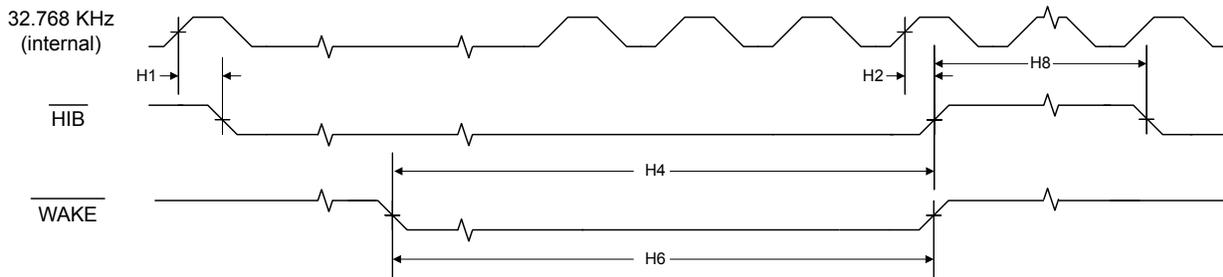
**Figure 25-16. V<sub>DD</sub> Ramp when Waking from Hibernation**
