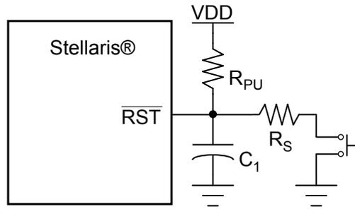
Typical  $R_{PU} = 10 \text{ k}\Omega$
