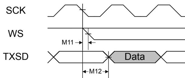
Figure 25-23. I<sup>2</sup>S Master Mode Receive Timing
