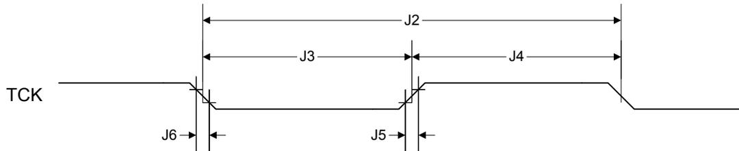
**Figure 25-9. JTAG Test Access Port (TAP) Timing**
