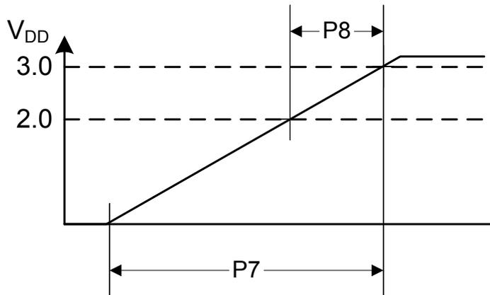
Figure 25-7. Voltage Requirements When Using an External V<sub>DCC</sub> Source
