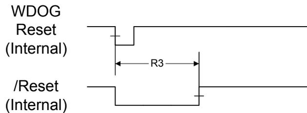
**Figure 25-13. MOSC Failure Reset Timing**
