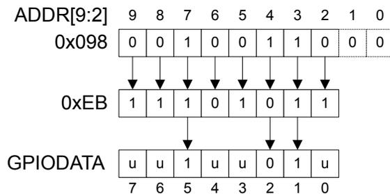
During a read, if the address bit associated with the data bit is set, the value is read. If the address bit associated with the data bit is cleared, the data bit is read as a zero, regardless of its actual value. For example, reading address GPIODATA + 0x0C4 yields as shown in Figure 9-4.
