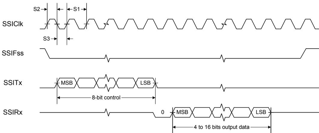
Figure 25-20. SSI Timing for SPI Frame Format (FRF=00), with SPH=1
