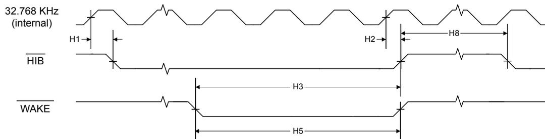
**Figure 25-15. Hibernation Module Timing with Internal Oscillator Stopped in Hibernation**
