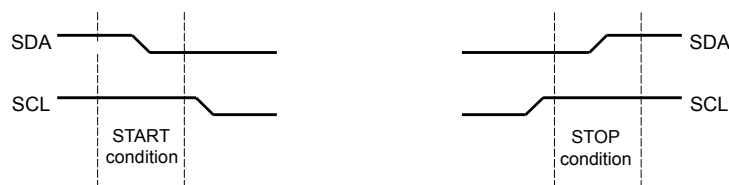
Figure 15-3. START and STOP Conditions
