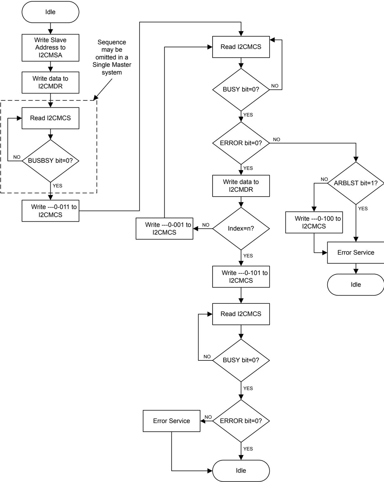
Figure 13-10. Master Burst RECEIVE
