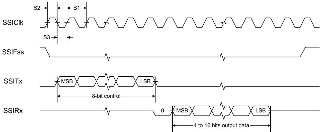
Figure 21-13. SSI Timing for SPI Frame Format (FRF=00), with SPH=1
