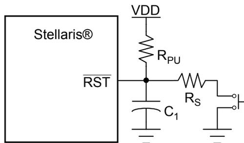
$$\text{Typical } R_{PU} = 10 \text{ k}\Omega$$
