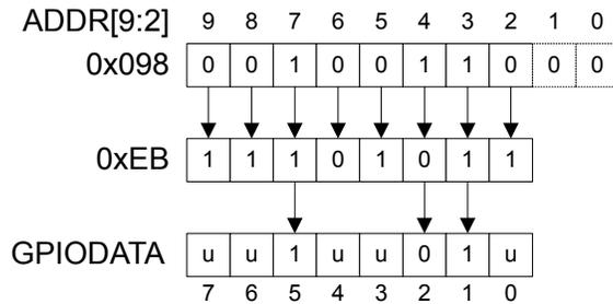
During a read, if the address bit associated with the data bit is set to 1, the value is read. If the address bit associated with the data bit is set to 0, it is read as a zero, regardless of its actual value. For example, reading address **GPIODATA** + 0x0C4 yields as shown in Figure 8-3 on page 291.
