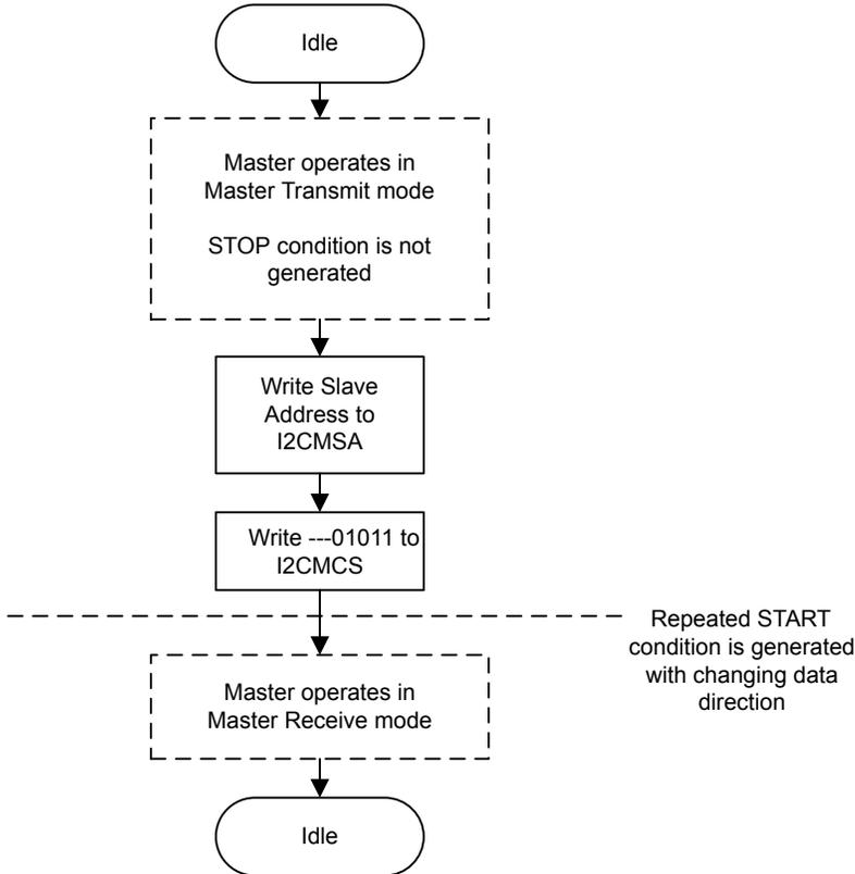
**Figure 13-12. Master Burst SEND after Burst RECEIVE**
