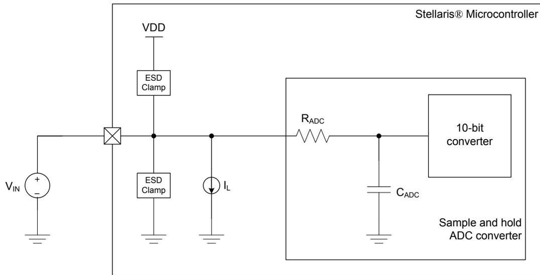
The ADC operates from both the 3.3-V analog and 1.2-V digital power supplies. The ADC clock can be configured to reduce power consumption when ADC conversions are not required (see “System Control” on page 187). The analog inputs are connected to the ADC through specially balanced input paths to minimize the distortion and cross-talk on the inputs. Detailed information on the ADC power supplies and analog inputs can be found in “Analog-to-Digital Converter (ADC)” on page 756.
