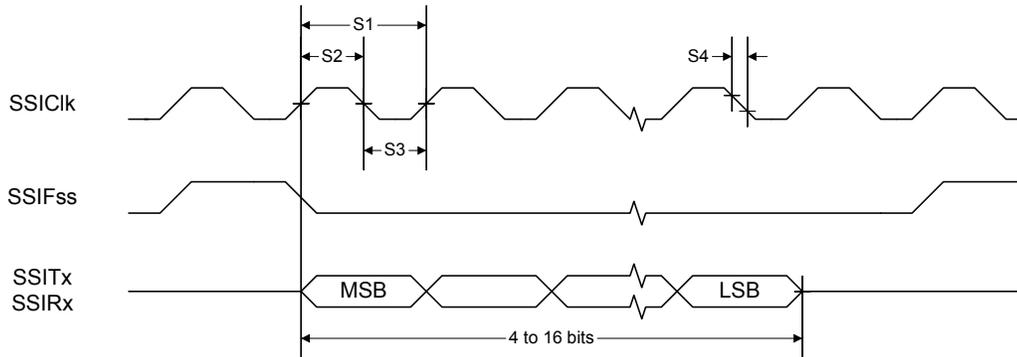
**Figure 20-15. SSI Timing for MICROWIRE Frame Format (FRF=10), Single Transfer**
