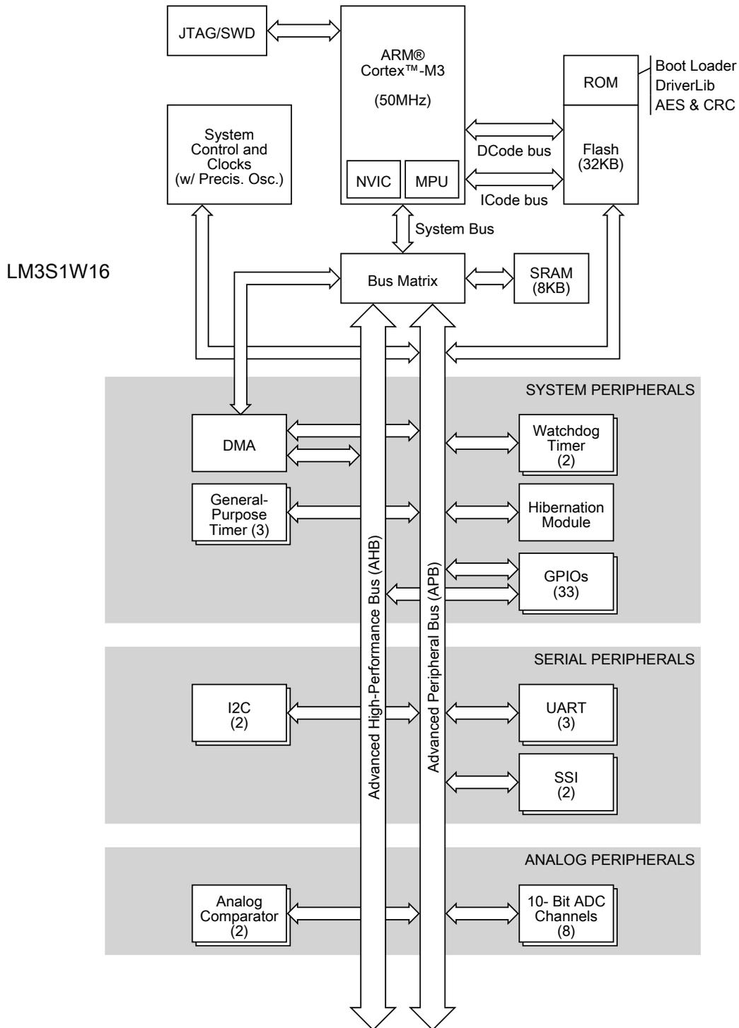
For applications requiring extreme conservation of power, the LM3S1W16 microcontroller features a battery-backed Hibernation module to efficiently power down the LM3S1W16 to a low-power state during extended periods of inactivity. With a power-up/power-down sequencer, a continuous time counter (RTC), a pair of match registers, an APB interface to the system bus, and dedicated battery-backed memory, the Hibernation module positions the LM3S1W16 microcontroller perfectly for battery applications.
