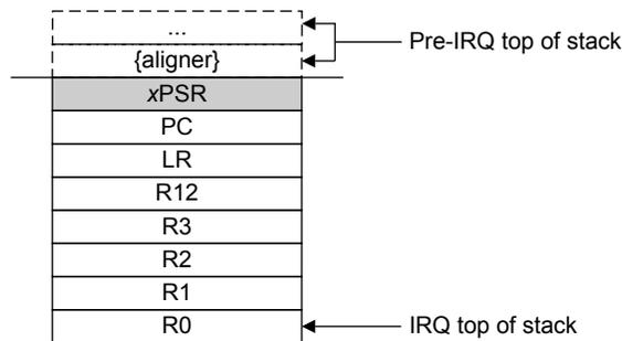
Immediately after stacking, the stack pointer indicates the lowest address in the stack frame.
