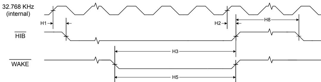
**Figure 20-12. Hibernation Module Timing with Internal Oscillator Stopped in Hibernation**
