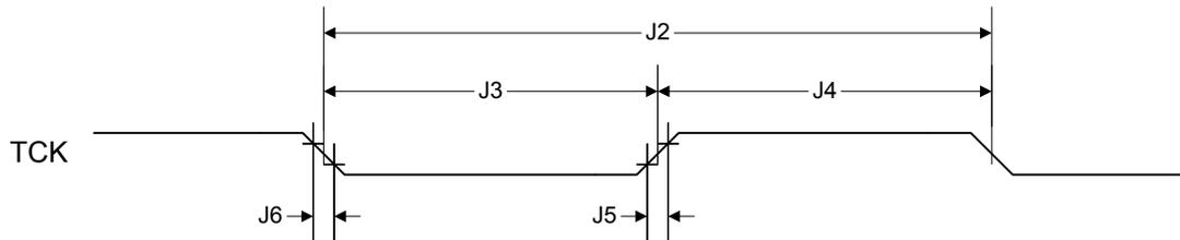
**Figure 20-3. JTAG Test Access Port (TAP) Timing**
