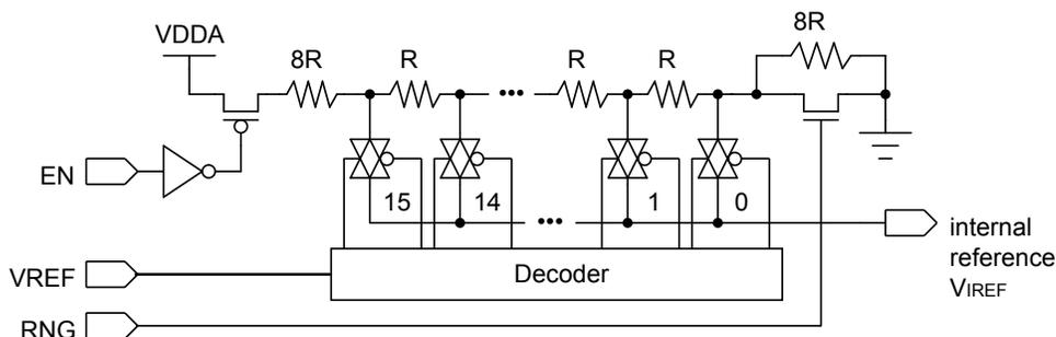
The internal reference can be programmed in one of two modes (low range or high range) depending on the `RNG` bit in the **ACREFCTL** register. When `RNG` is clear, the internal reference is in high-range mode, and when `RNG` is set the internal reference is in low-range mode.
