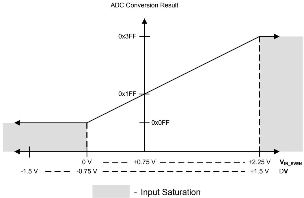
Figure 12-9. Differential Sampling Range,  $V_{IN\_ODD} = 2.25\text{ V}$
