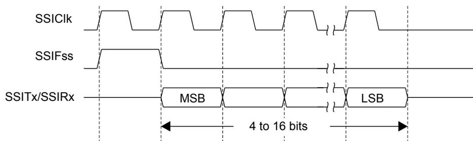
In this mode,  $SSIClk$  and  $SSIFss$  are forced Low, and the transmit data line  $SSITx$  is tristated whenever the SSI is idle. Once the bottom entry of the transmit FIFO contains data,  $SSIFss$  is pulsed High for one  $SSIClk$  period. The value to be transmitted is also transferred from the transmit FIFO to the serial shift register of the transmit logic. On the next rising edge of  $SSIClk$ , the MSB
