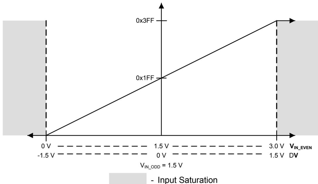
Figure 12-8. Differential Sampling Range,  $V_{IN\_ODD} = 0.75\text{ V}$
