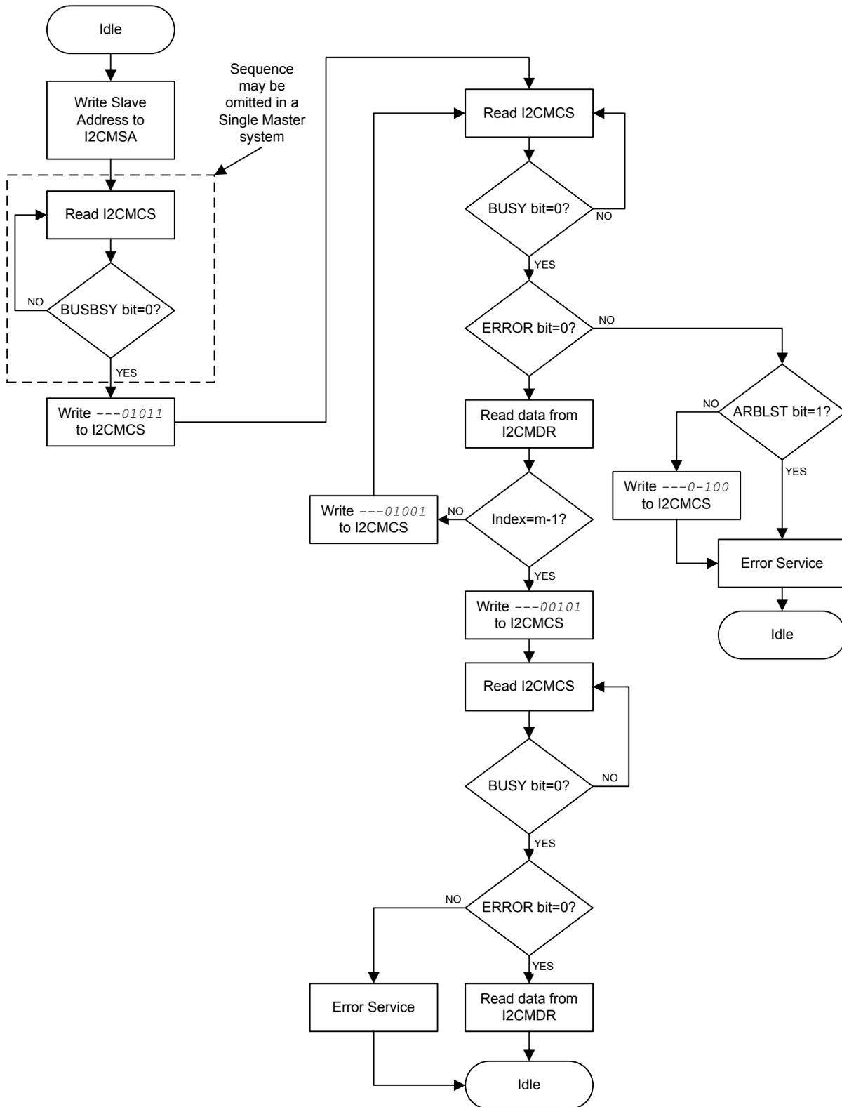
Figure 15-11. Master RECEIVE with Repeated START after TRANSMIT with Repeated START
