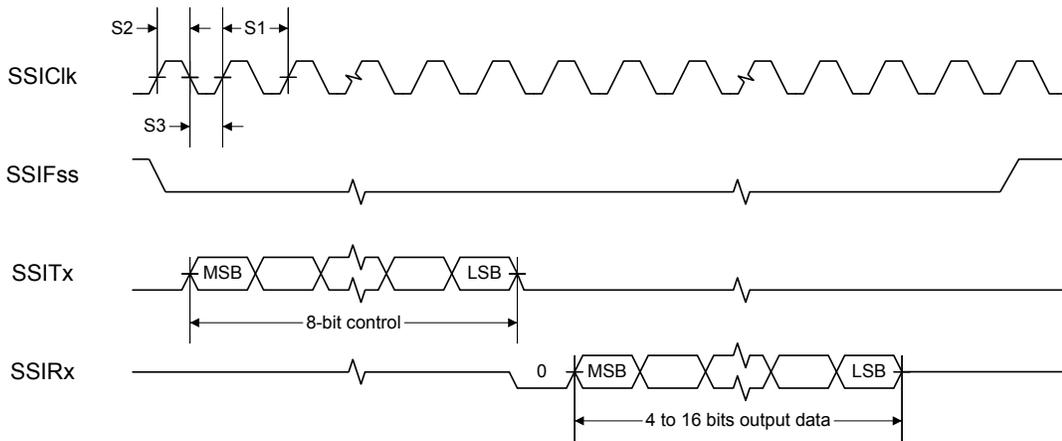
Figure 20-16. SSI Timing for SPI Frame Format (FRF=00), with SPH=1
