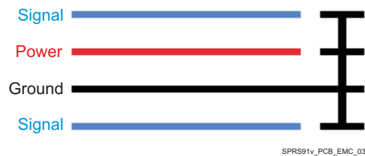
Figure 7-13. Guard Ring Routing
