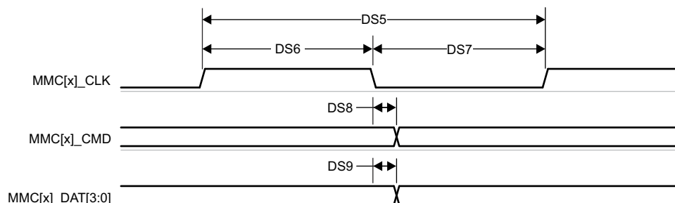
Figure 6-87. MMC1/2 – Default Speed – Transmit Mode
