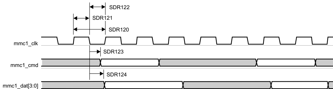
Figure 7-65. MMC/SD/SDIO in - High Speed SDR12 - Transmitter Mode
