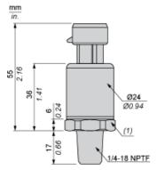
(1) SW24 tightening torque ≤ 25 N.m / 221 lb-in
