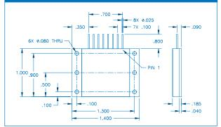
The UDOS001 drawing shows the hermetic package, mounting flange and 8 external connections. All dimensions given are in inches and tolerances are  $\pm 0.005$ . The package walls are 0.040 inch thick and the cover is 0.010 inch thick.
