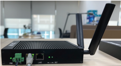
Figure 9.2 Connecting an Ethernet cable to the GW66.
