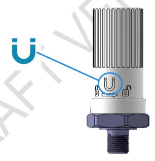
The magnet must be of sufficient strength and proximity to create a magnetic field of 25 mT at the switch location.
