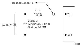
Note: Input reflected-ripple current is measured with a simulated source impedance of 12 µH. Capacitor Cs offsets possible battery impedance. Current is measured at the input of the module.
