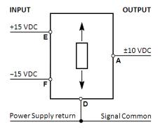
A through F: Connector pin assignments
