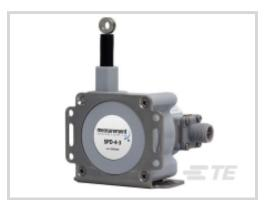
Position Sensor Product Type: SP Series, String Pots Full Stroke Range: 1270 mm [ 50 in ] Output Signal Type: 0 – 10 VDC, 4 – 20 mA Accuracy: ±.25 % of FS Repeatability: .02 % of FS All Compact String Pot, User Select Output (4)
