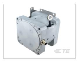
Position Sensor Product Type: SK Series, IP67 String Pots Full Stroke Range: 10160 mm [ 400 in ] Output Signal Type: Voltage Divider (Potentiometric) Accuracy: ±.35 % of FS Repeatability: .02 % of FS
