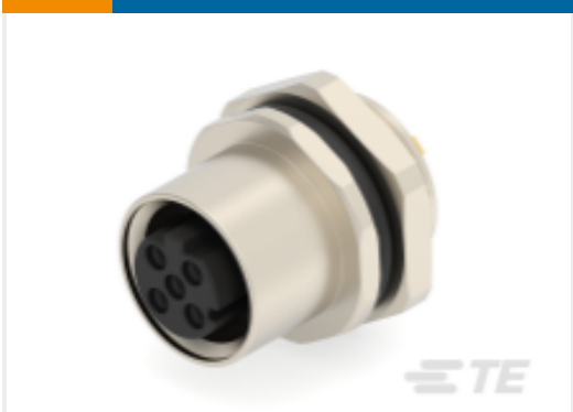
TE Part #T4133512041-000 M12,FRONT MOUNT,FEMALE,D,4P, SOLDER WIRE
