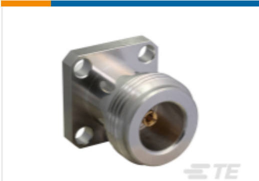
TE Part #CONN002-W N Type Jack 50 Ohm Panel Mount
