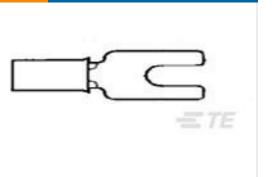
TE Part #40521 SPADE TERMINAL 18-14 AWG TPBR
