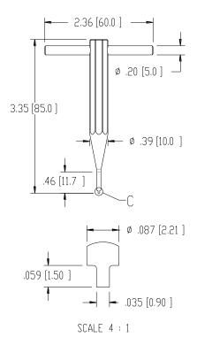
WRENCH TOOL (MEAS P/N IC-D00546) FOR PRODUCT W/o FITTING. TOOL CAN BE ORDERED SEPARATELY FROM MEAS.
