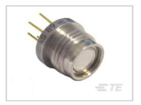
Pressure: **[ 5000 psi ]** Pressure Sensor Type: **mV Output Pressure Sensors** Pressure Type: **Absolute** Output Signal Type: **Sensitivity = 15 - 28mV/V** Supply Voltage Range: **5 V**
