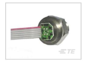
Pressure: **[ 3000 psi ]** Pressure Sensor Type: **mV Output Pressure Sensors** Pressure Type: **Sealed Gauge** Output Signal Type: **125 mV** Operating Temperature Range: **-40 – 125 °C [ -40 – 257 °F ]**
