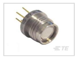
Pressure: **[ 3000 psi ]** Pressure Sensor Type: **mV Output Pressure Sensors** Pressure Type: **Absolute** Output Signal Type: **Sensitivity = 15 - 28mV/V** Supply Voltage Range: **5 V**
