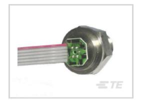
Pressure: [1000 psi] Pressure Sensor Type: mV Output Pressure Sensors Pressure Type: Absolute Output Signal Type: 125 mV Operating Temperature Range: -40 – 125 °C [-40 – 257 °F]
