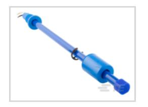
Entry Style: Bottom, Top Fluid Type: Alcohol, Fuel, Oil Contact Form: A+B Port Fitting: M16 External, M16 Internal Case Material: Glass Filled Nylon 6.6
