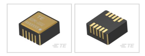
Acceleration Range (±): 500 g Frequency Response: 2 to 10000 Hz Overall Acceleration Range (±): 500 g Accelerometer Type: 3-Wire Voltage Number of Axes: 1
