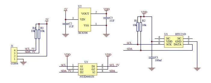
Connector Pin Assignments (I<sup>2</sup>C Communications)
