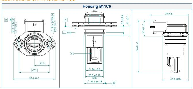
Recommended Screw Mounting: M6; Typical tightening torque: 12 N.m; Maximum tightening torque: 17 N.m
