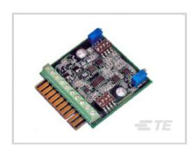
Voltage Requirements: -15 - 15 VDC, -12 - 12 VDC
