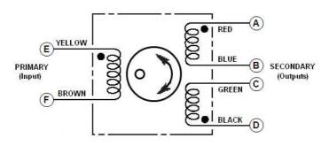
A through F: Connector pin assignments; Connect B to C for differential output
