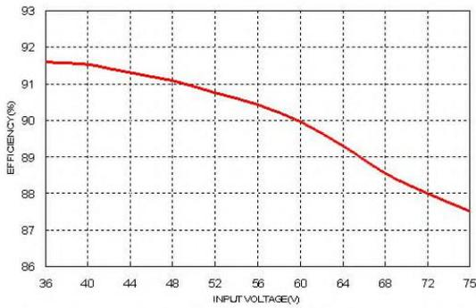
Efficiency Versus Input Voltage, Full Load
