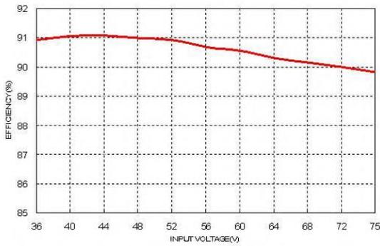
Efficiency Versus Input Voltage. Full Load
