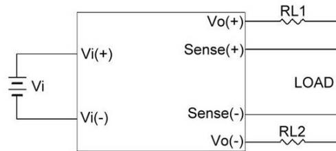
Operation Output Voltage with Sense Function Used
