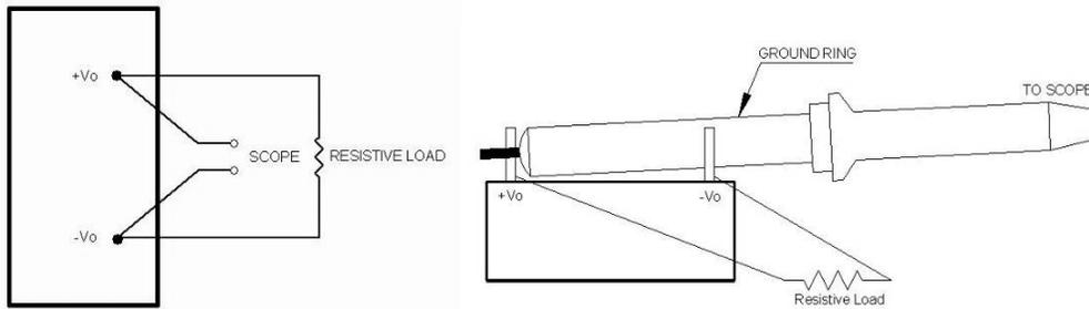
Output voltage and efficiency measurement test
