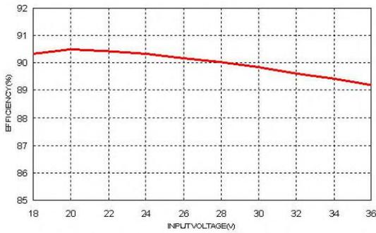
Efficiency Versus Input Voltage. Full Load
