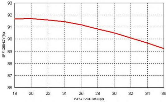
Efficiency Versus Input Voltage. Full Load
