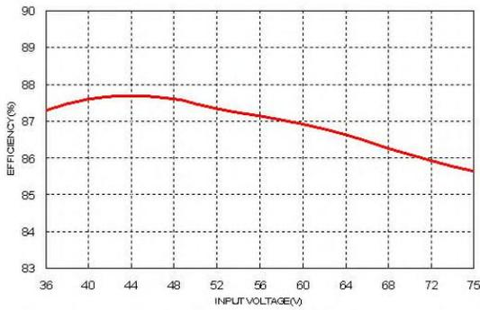
Efficiency Versus Input Voltage. Full Load
