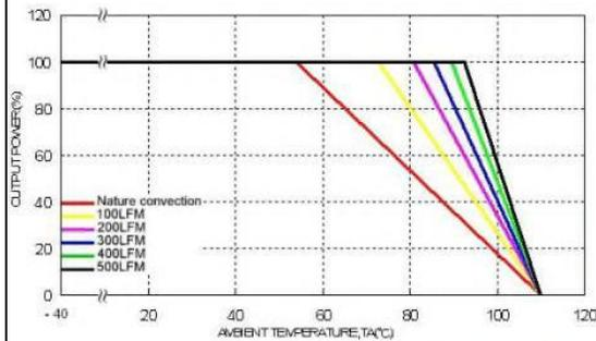
Derating Output Current Versus Ambient Temperature with Heat-Sink and Airflow V<sub>in</sub> = V<sub>in</sub>(nom)
