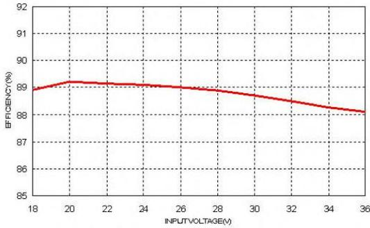
Efficiency Versus Input Voltage. Full Load
