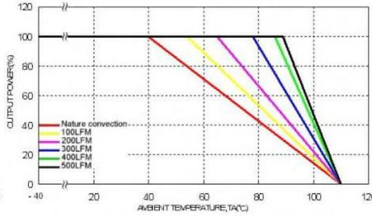
Derating Output Current Versus Ambient Temperature and Airflow V<sub>in</sub>=V<sub>in</sub>(nom)
