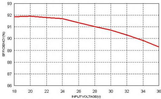
Efficiency Versus Input Voltage. Full Load
