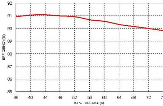
Efficiency Versus Input Voltage. Full Load
