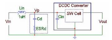
Figure C: NQ12 converter with Input Filter
