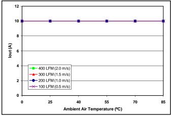
Figure 9: Maximum output power derating curves vs. ambient air temp for 3.3Vo, 5.0Vo units. Airflow rates of 100 - 400 LFM with air flowing across the converter from pin 11 to pin 1 (Vin nom, vert mount).
