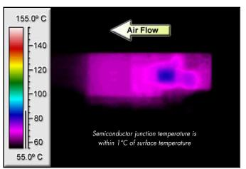
Figure 6: Thermal plot of 0.9Vo, 1.2Vo, 1.5Vo converters at 10 amp load current with 55°C air flowing at the rate of 200 LFM. Air is flowing across converter from pin 11 to pin 1 (Vin nom, vert mount).
