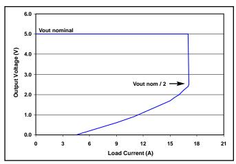
Figure 4: Output voltage vs. load current showing current limit inception point and fold-back current limit behavior.
