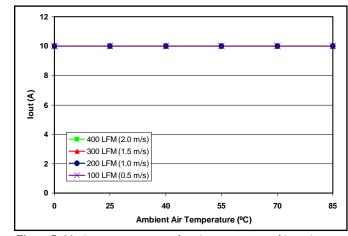
Figure 7: Maximum output power derating curves vs. ambient air temp for 1.8Vo, 2.5Vo units. Airflow rates of 100 - 400 LFM with air flowing across the converter from pin 11 to pin 1 (Vin nom, vert mount).
