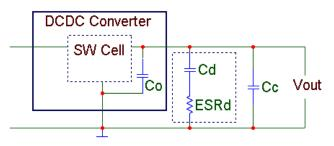
Figure F: Converter with Additional Output Capacitance
