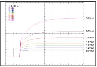
Figure 12: Turn-on transient at zero load (500 µs/div). Ch 1: ON/OFF input (5V/div) Ch 2-8: Vout (1V/div)
