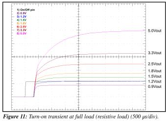
Ch 1: ON/OFF input (5V/div) Ch 2-8: Vout (1V/div)
