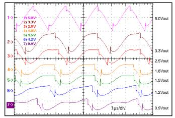
**Figure 17:** Input Terminal Ripple Voltage at nominal input voltage and rated load current (200 mV/div). Load capacitance:  $10\mu F$  ceramic cap. Bandwidth: 20 MHz. See Figure 15.
