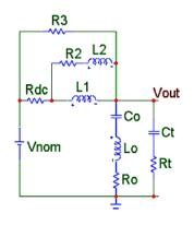
Figure D: NQ12 Passive Output Model
