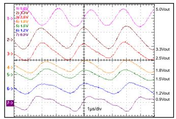
**Figure 16:** Input Reflected Ripple Current,  $i_{S}$  through a 1  $\mu$ H source inductor at nominal input voltage and rated load current (50 mA/div). See Figure 15.
