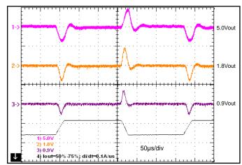
Figure 13: Output voltage response for 0.9V, 1.8V, 5.0V units to step-change in load current (50-75-50% of Iout max; di/dt=0.1A/ $\mu$ s). Load cap: 15 $\mu$ F, 100m $\Omega$  ESR tant, 10 $\mu$ F cer. Ch 1: Iout (5A/div), Ch 2-4: Vout (100mV/div).
