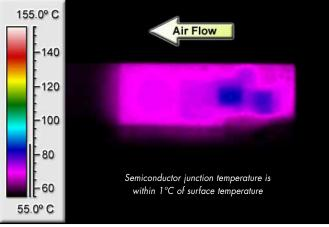
*Figure 8:* Thermal plot of *1.8Vo*, *2.5Vo* converters at 10 amp load current with 55°C air flowing at the rate of 200 LFM. Air is flowing across converter from pin 11 to pin 1 (Vin nom, vert mount).
