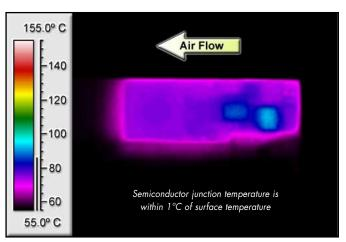
Figure 10: Thermal plot of 3.3Vo, 5.0Vo converters at 10 amp load current with  $55^{\circ}C$  air flowing at the rate of 200 LFM. Air is flowing across converter from pin 11 to pin 1 (Vin nom, vert mount).
