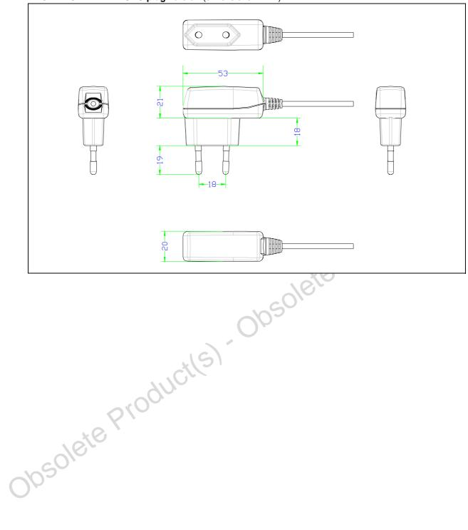
MECHANICAL DATA EURO plug version (dimensions in mm)
