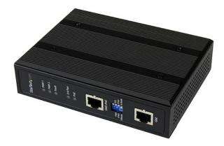
The POEINJ1GI Industrial Gigabit PoE+ Injector provides power and data connectivity to a Gigabit PoE-compliant device over standard Ethernet cabling at distances of up to 330ft (100m), and offers redundant, wide-range DC power inputs. This injector allows you to easily connect a PoE-powered device (PD) to a non-PoE LAN switch, avoiding the cost of upgrading your switch to a PoE-enabled model.
