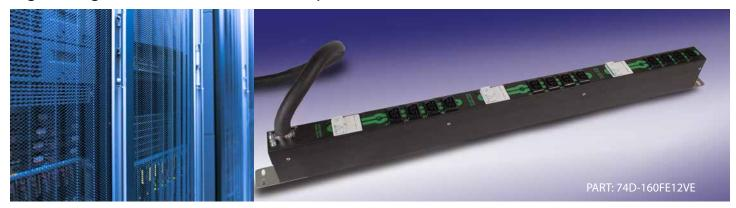
The API Technologies 380VDC Rack Mount Power Strips are designed to be hard wired into the main power infrastructure and provide a total of 30A or 60A of power via Anderson Power Products connectors. The outlets are divided up into load banks containing a choice of outlets based on size and are protected by a choice of fuses or UL1077 breakers.
