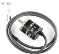
This 200 pulse per rotation rotary encoder outputs gray code which you can interpret using a microcontroller and find out which direction the shaft is turning and by how much. This allows you to add feedback to motor control systems. Encoders of this kind are often used in balancing robots and dead reckoning navigation but it could also be used as a very precise input knob. The encoder comes with a set screw coupler which will attach to any 4mm shaft.
