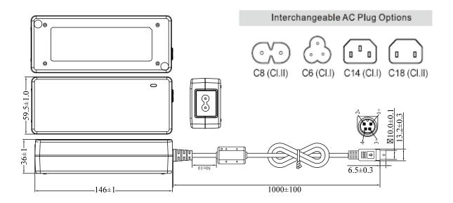
DC Cable: UL1185 16AWG 1000 mm with ferrite core Connector: #03 -  $2.5 \times 5.5 \times 9.5$  mm, fork type, 18 to 52 V #49 - 4PIN (Keycon equal), 12 to 17 V
